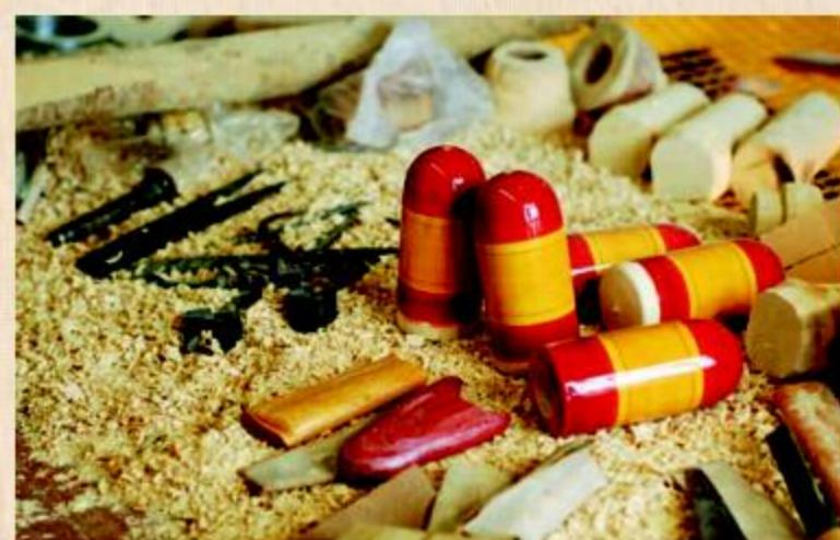
The tools and manufacturing process are traditional but the method is now mechanised and the lathes are machine-powered. As the wood spins, it is shaped using a variety of tools. Natural pigments are melted with lac into coloured sticks, which are pressed against the rotating wood. As the lac melts, the colour is transferred onto the surface. Some artisans have learnt this technical skill from their ancestors. Others received government training aimed at reviving this handicraft tradition.
